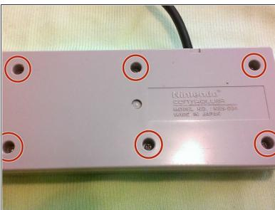
Remove the 6 8mm screws in the back cover using a #1 Philips screwdriver.
