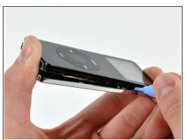
Repeat the same procedure listed in the previous step to free the five clips along the headphone jack side of the iPod.
