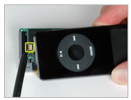
Use a spudger to flip up the black plastic tab holding the orange click wheel ribbon in place. The black tab will rotate up 90 degrees, releasing the ribbon cable.
