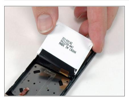
Lift the display up and out of the iPod.
