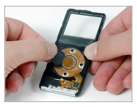
Push the click wheel button through from the front side of the iPod and lift it out of the iPod.
