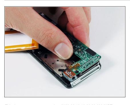
Gently lift up on the dock connector end of the logic board to ensure the logic board is free.
