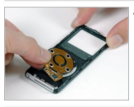
Lift the click wheel out of the front panel.
