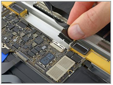
Disconnect the display cable by gently pulling it straight out of its connector.
