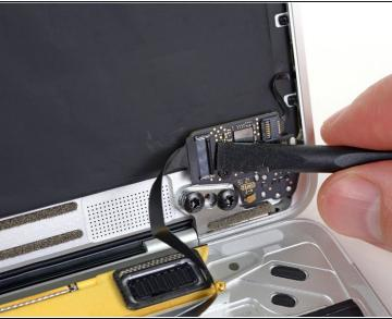
• Use a spudger to flip open the retaining flap on the audio jack board cable ZIF connector.
