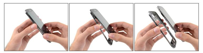
• Remove the midframe from the display assembly.
