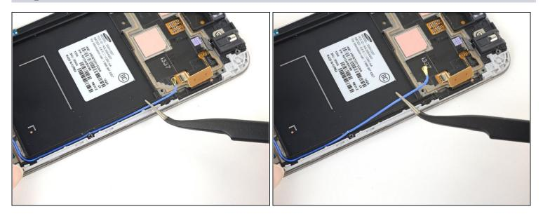
• Use tweezers to lift and de-route the antenna cable from the edge of the case.
