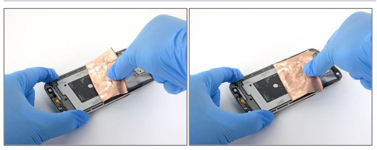
Grab the foil liner underneath the LCD and peel it away from the case.
