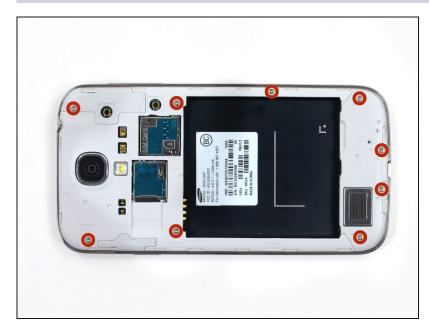
Remove the nine 4.0 mm Phillips #00 screws securing the midframe to the display assembly.
