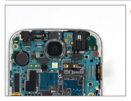
• Remove the single 2.4 mm Phillips #00 screw from the motherboard assembly.
