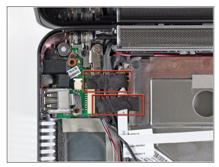
ilf present, remove the two pieces of tape covering the cables routed near the USB and power board.
