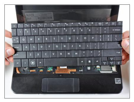
Lift the keyboard out of the upper case, minding the cable that is still connecting it to the motherboard.
