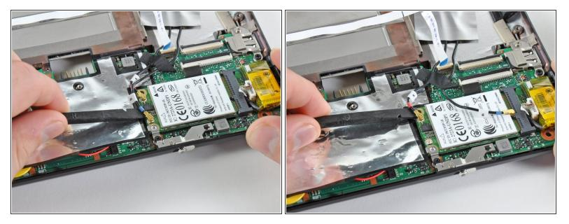
Use the flat end of a spudger to pry both antenna connectors up from their sockets on the Wi-Fi board.
