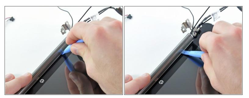
Use the edge of a plastic opening tool to pry the left side of the speaker grill away from the display assembly.
