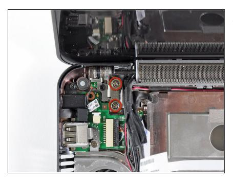
Remove the two 5 mm Phillips screws securing the left display hinge to the lower case.
