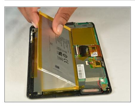
Lift the battery from the device.
