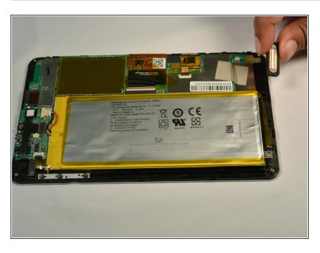
Lift the speaker away from the device and replace it with the new one.
