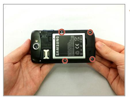
Remove the four 3.8mm Phillips #000 screws securing the back assembly to the phone.
