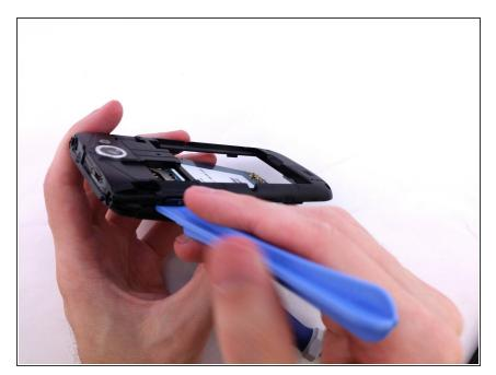
With plastic opening tool continue prying around the edge of the back assembly.
