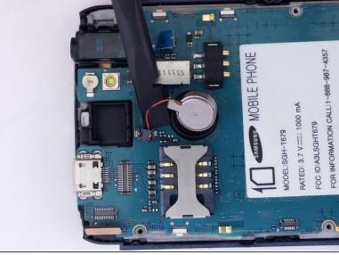
Use the flat end of a spudger to remove vibrator cable from motherboard.
