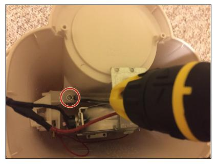
• Remove the 7mm Phillips screw from the power button.
