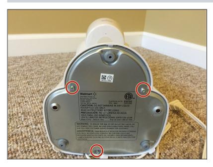
Locate and unscrew the 3 8mm
