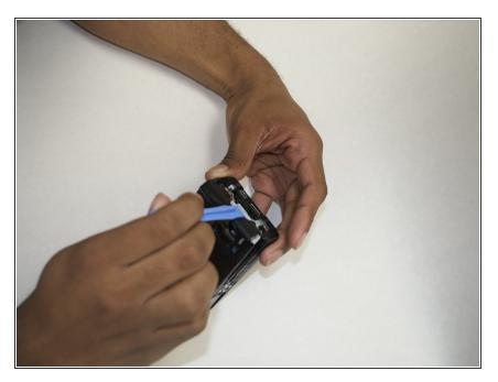
Once the screws are removed, use a spudger to carefully detach the cover.
