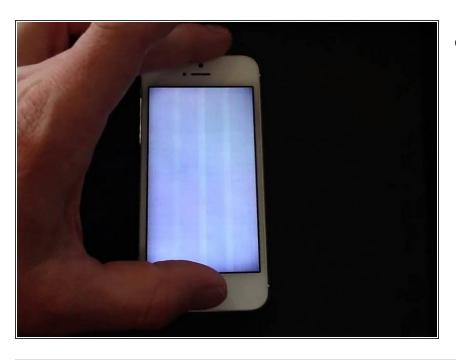
The display has an IC that could be damaged. Check particularly on the upper left and right corners. Any signs of damage indicate the part is defective and needs to be replaced with a new one.
