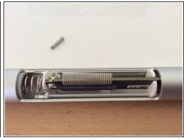
Now remove that one little philips screw, holding the logic board assembly in place.
