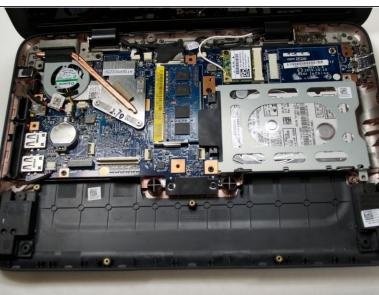
• Lastly, remove the white power connector that attaches the battery to the motherboard (to make this easier to see, the power connector is outlined in red in the photograph). Now remove the battery from the device and place to the side.
