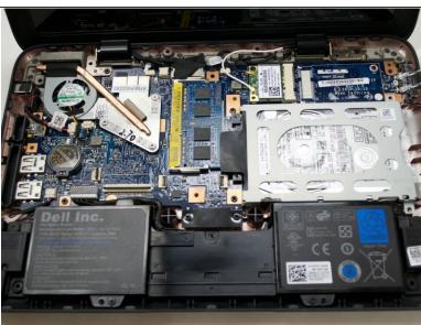
Next, remove the top cover from the device using the plastic opening tools. It snaps in on the sides, so don't worry if you hear it unsnapping; it's not breaking.
