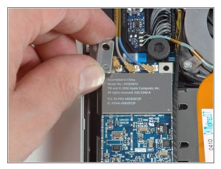
Lift the small silver metal retaining bracket up and out of the computer.
