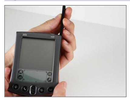
Remove the stylus from the side of the PDA by sliding it upwards.
