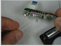
Remove the plastic flash cover using a spudger.
