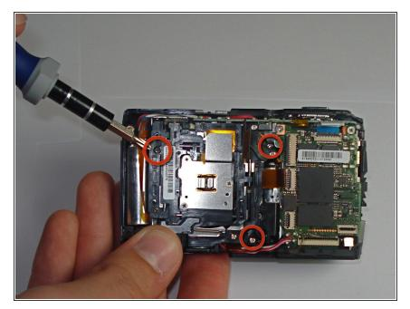
Remove the three screws from the inside of the camera using a #00 screwdriver.
