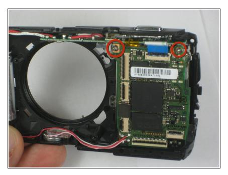
Remove the two Phillips #00 screws on the right side of the camera.
