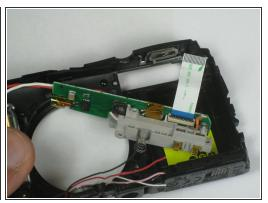
Pull gently on the white tab to remove the small motherboard with the flash device on it.
