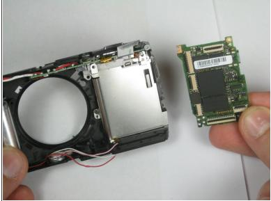
In order to remove the motherboard, grab each side of it and pull up using your thumb and forefinger.
