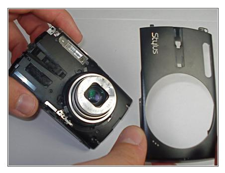
Remove the black front panel by sliding it towards the lens and then pulling it up off of the camera.
