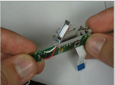
Remove the flash bulb using a plastic spudger.
