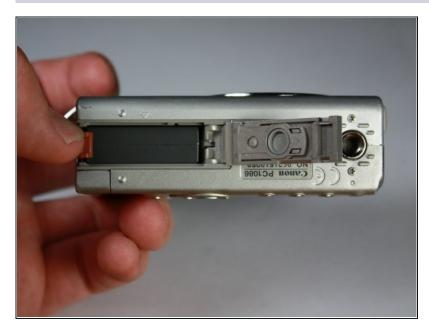
• Pull the orange lever and the battery will spring out slightly.
