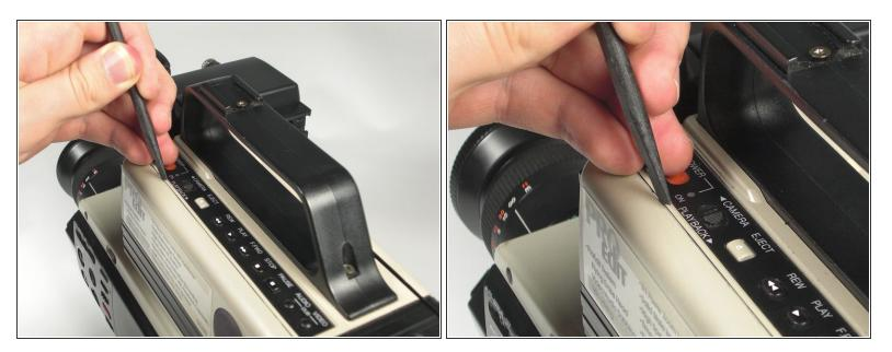
• Pry along the seam on the top side near the buttons with a spudger.
