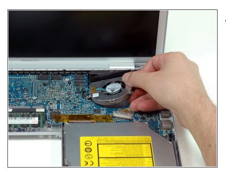
Lift the right fan up and carefully peel up the tape securing the fan to the heat sink as you go.
