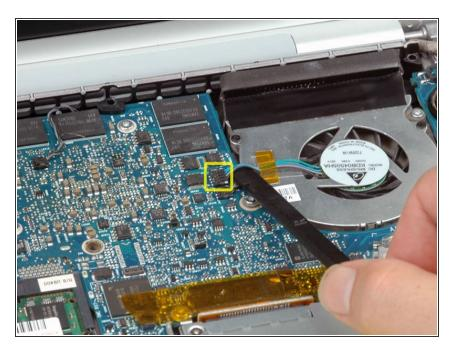
Disconnect the right fan cable from the logic board by placing a spudger beneath the cable and lifting up.
