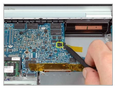
Disconnect the right thermal sensor cable from the logic board by placing a spudger beneath the cable and lifting up.
