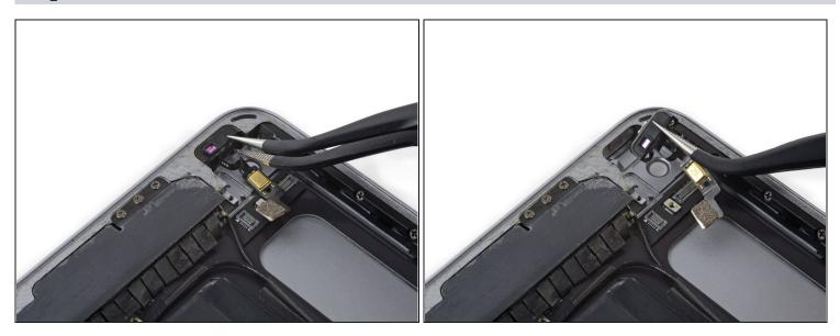
Remove the power button assembly.
