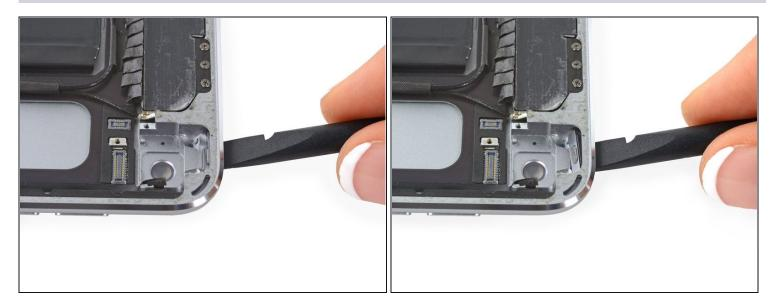
• Use a spudger to press the power button into the iPad and remove it.
