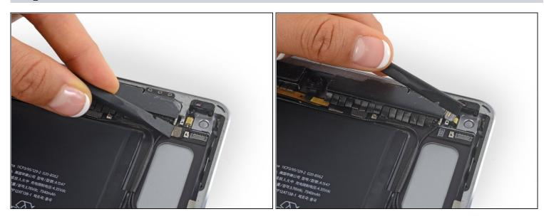
• Use the flat end of a spudger to pry up the power button/microphone ribbon cable connector from its socket.
