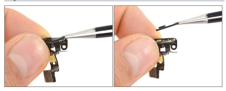
• Flip the assembly over and peel up the black rubber piece covering the portion of the ribbon cable with the ambient light sensor.
