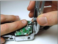
• With the spudger, pry back the cover starting with the outer edge to release.
