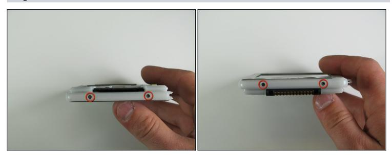
• Remove the four 2.6 mm Philips screws on the top and bottom of the frame.
