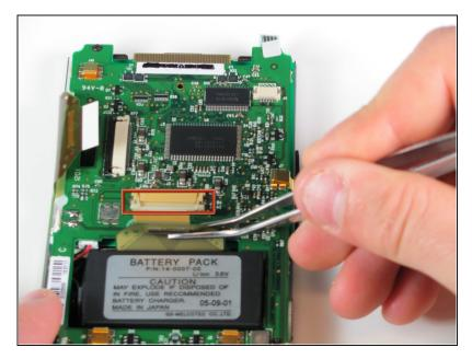
Using the same technique as with the other ribbons, locate and remove the ribbon cable above the battery pack.
