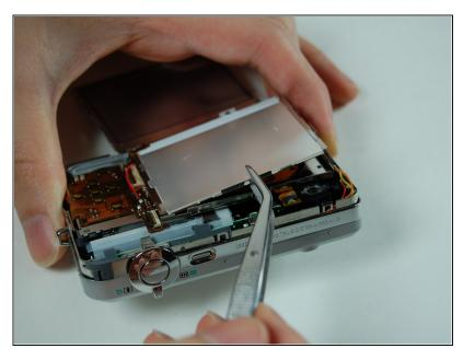
• Use your tweezers to lift the LCD frame from the camera.
