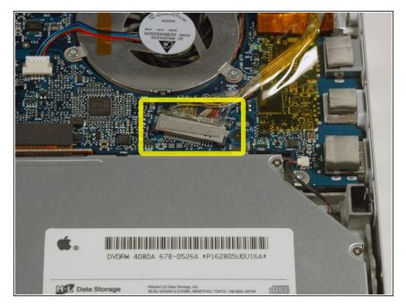
Disconnect the display data cable from the logic board.
