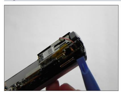
Next, use a plastic removal tool and separate the silver front case from the black frame.
