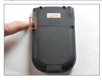
While sliding the silver release tab up, simultaneously lift the cover up from the left side.
