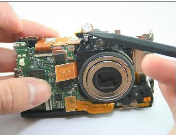
• Use spudger to carefully lift the LED light off the upper-left corner of the lens.
