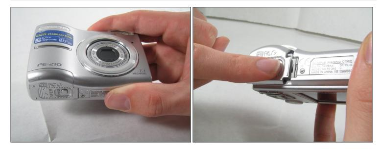
• The battery compartment is located on the bottom side of the camera. Push the button in, and slide the cover to get access to the batteries.
