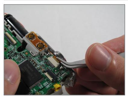
Remove the ribbon cord located near the top right corner of the motherboard. Do this by carefully pulling the cord out of the socket using a pair of tweezers.
