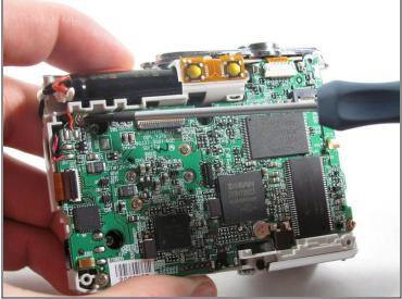
Remove the seven 2.7 mm using a #00 screwdriver.
