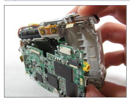
• Remove the motherboard from the camera casing.
