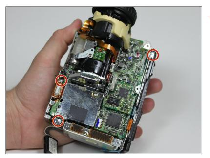
Remove the three screws from the circuit board.
