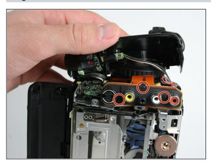
Remove the three 4.5 mm screws from the right face of the video camera.
