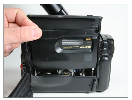
Pull off the plastic tape cover by lifting it up and out of the camera base.
