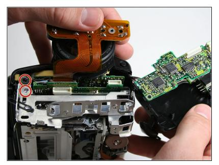
Remove two remaining 3.6 mm case screws from the front of the camera.
