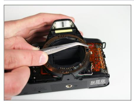
• Use a pair of <u>tweezers</u> to remove the spring on the lens mounting ring.
