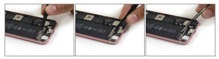
• Use <u>tweezers</u> to peel up the edges of the two adhesive strips at the bottom of the battery.
