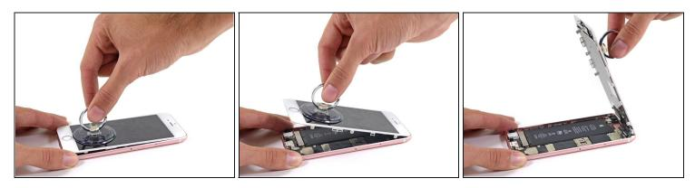
• Use the suction cup to open the display, breaking the last of the adhesive.
