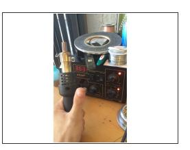
Disassemble to get to motherboard of device, wrap with kapton tape to avoid damaging any other components. Take heatgun and heat old port
