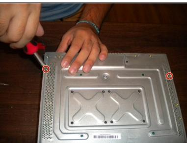
Place the console with the metal side facing you and take your multi-screwdriver (using the star head) and remove the six screws labeled in the picture below
