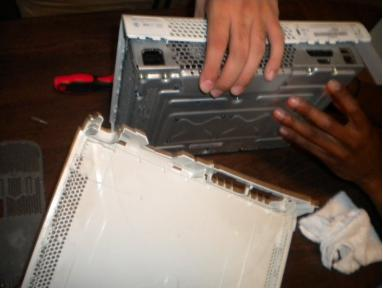
● Take the tweezers, or pliers, and poke the seven holes that are visible to you. Remove the cover.
