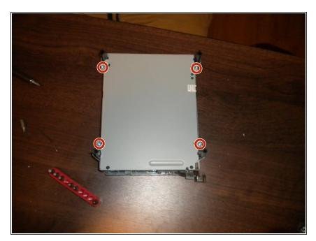
Place the box so the bottom is facing up. Remove the four screws labeled in the picture below with a multi-screwdriver with the five-point head.
