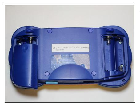
• Remove the battery covers and the four batteries.
