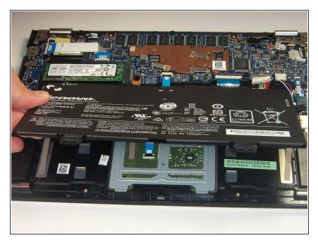
Carefully remove the battery from the device.
