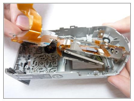
• Remove LCD plate to expose LCD components and ribbon cables
