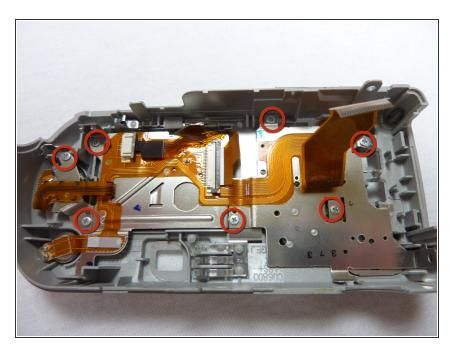
• Remove 7 Screws to remove plate and expose LCD screen.
