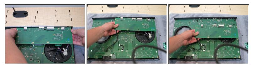
For this step, grab both sides of the sound card and carefully bring it straight up for removal. There are small metal prongs on the bottom of the sound card that connect with the motherboard. To eliminate the possibility of damaging the prongs, it is pertinent that the sound card is not removed on an angle.
