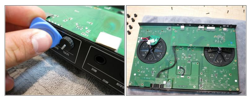
Before removing the sound card, the 2 gain knobs in the back of the unit will need to be removed.
