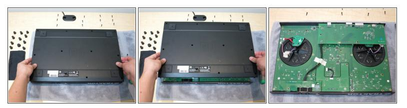
Next, remove the back plate of the controller. Simply grab the edges of both ends of the controller and lift up.
