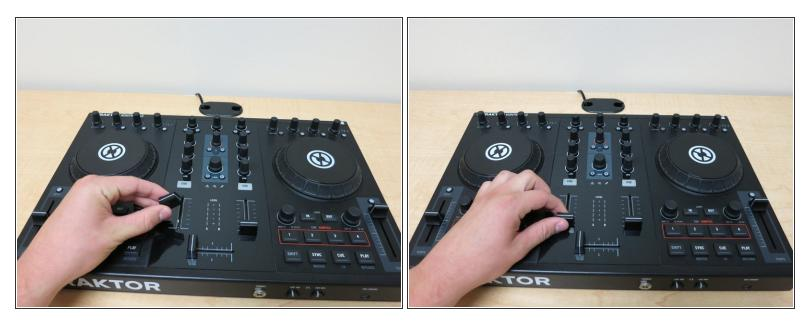
Carefully, place the tempo faders, channel fader, and the cross fader, back on to controller in its correct spot.
