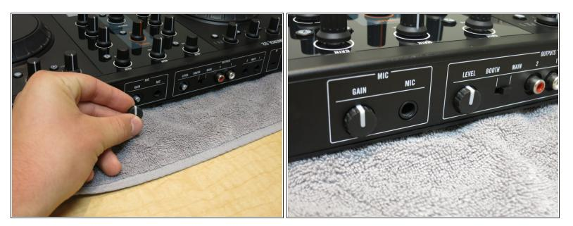
Finally, place the gain knobs back on to the rear of the controller. Be sure to push each knob in until they click and feel snug.
