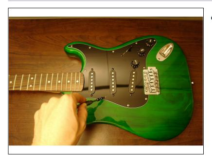
• With a screwdriver, remove the front body perimeter screws.
