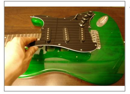
• Carefully lift the panel of the guitar and turn it upside down to reveal the electronic components.
