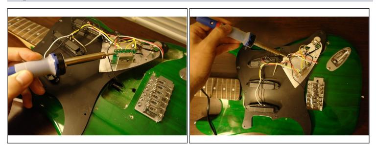
• Using the the soldering iron and the <u>solder sucker</u> (or the soldering wick), take away any soldering connections of the potentiometers and the five-way switch.
