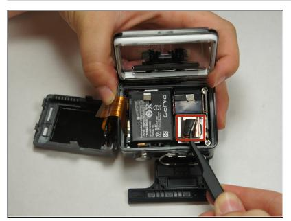
Using <u>tweezers</u>, peel off the copper tape on the right side of the battery.
