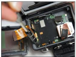
• Remove the three 4 mm Phillips #000 screws securing the motherboard.
