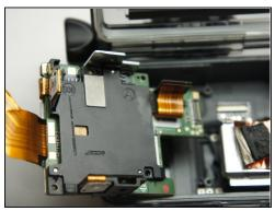
• Use your fingers and carefully pull out the motherboard from under the lens. It may take a little bit of adjusting to get it out.
