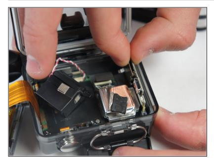
Gently lift the microSD/Micro USB assembly up and out of the device.
