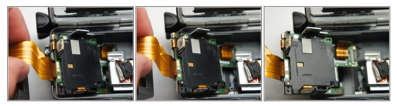
• Use your fingers and carefully pull out the motherboard from under the lens. It may take a little bit of adjusting to get it out.
