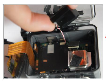
• Use your fingers and gently pull out the sensor from the motherboard by slowly and gradually pulling up on the image sensor box.
