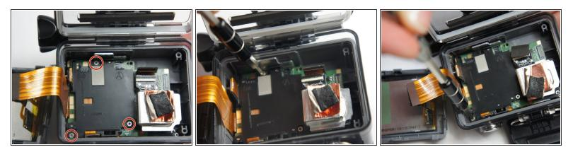
• Remove the three 4 mm Phillips #000 screws securing the motherboard.
