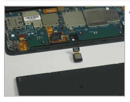
Carefully remove the front camera from the device.
