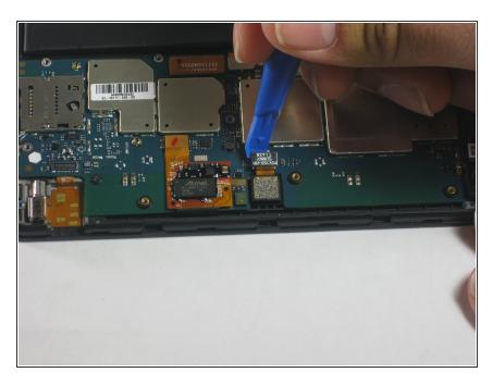
Use a plastic opening tool to gently disconnect the front-facing camera from the motherboard.
