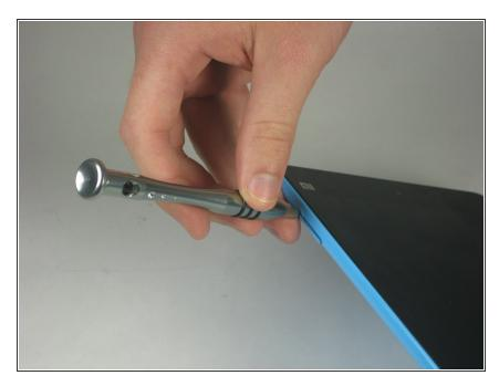
Remove the micro SD card slot from the left side of the device using either the metal pin included with the device or a SIM card eject tool.
