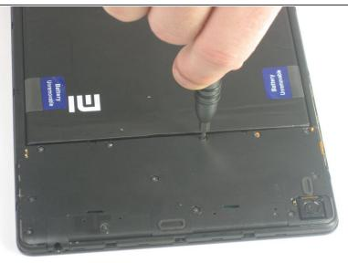
Remove the twelve 3.0 mm Phillips #000 screws on the upper cover of the device.
