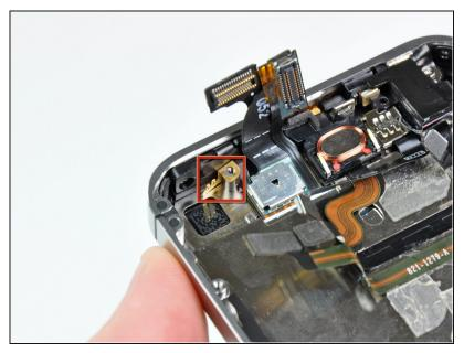
⚠ Be sure not to lose the small grounding finger for the rear facing camera near the power button.
