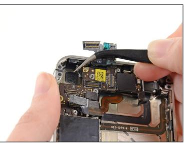
② If present, remove the piece of tape covering a Phillips screw near the power button.
