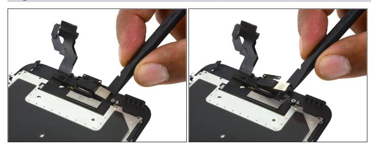
• Use the flat end of a spudger to lift the FaceTime camera out of its housing.
