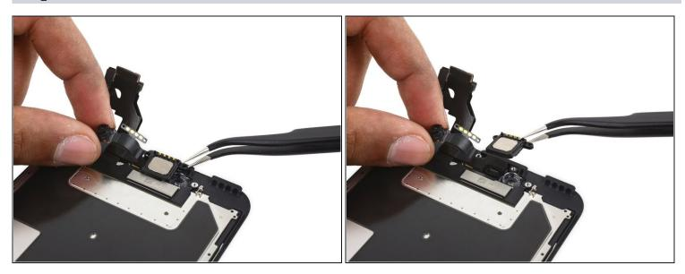
• Pull the FaceTime camera back and remove the earpiece speaker.
