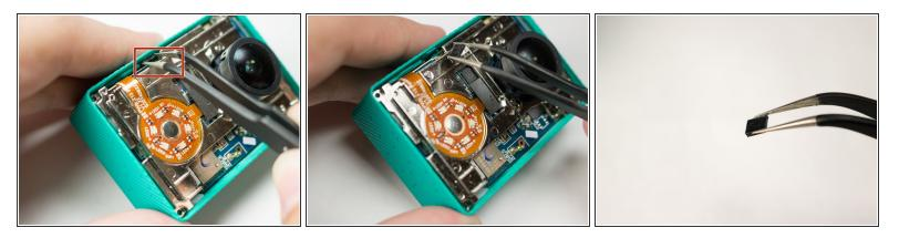
Pull on and remove the black spacer located at the top inside of the camera body using the tweezers and set the part aside.
