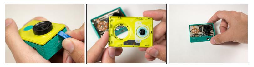
• Slide prying tool along the seam until front panel is fully separated from the back panel.
