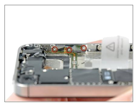
Remove the three 1.6 mm Phillips screws securing the volume button bracket to the outer case.
