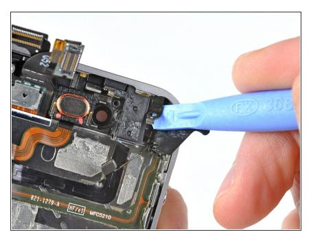
Use the edge of a plastic opening tool to gently move the top antenna contact away from the headphone jack.
