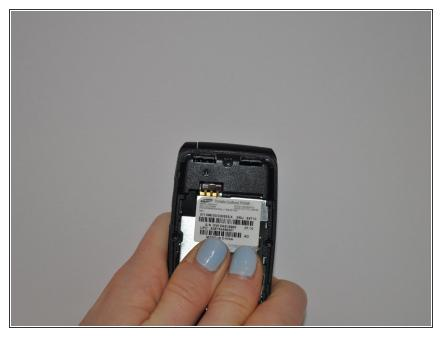
Remove the battery by pressing the battery lock down and slide the battery cover away.
