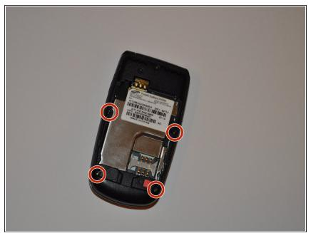
Locate the 4 screws holes on the phone and remove them with the #000 Philips Head screwdriver. (See red circles)
