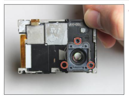
Remove the three 8 mm Phillips #000 screws securing the lens.
